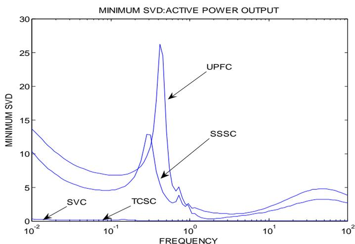
Figure 7: Minimum SVD for Active Power Feedback
