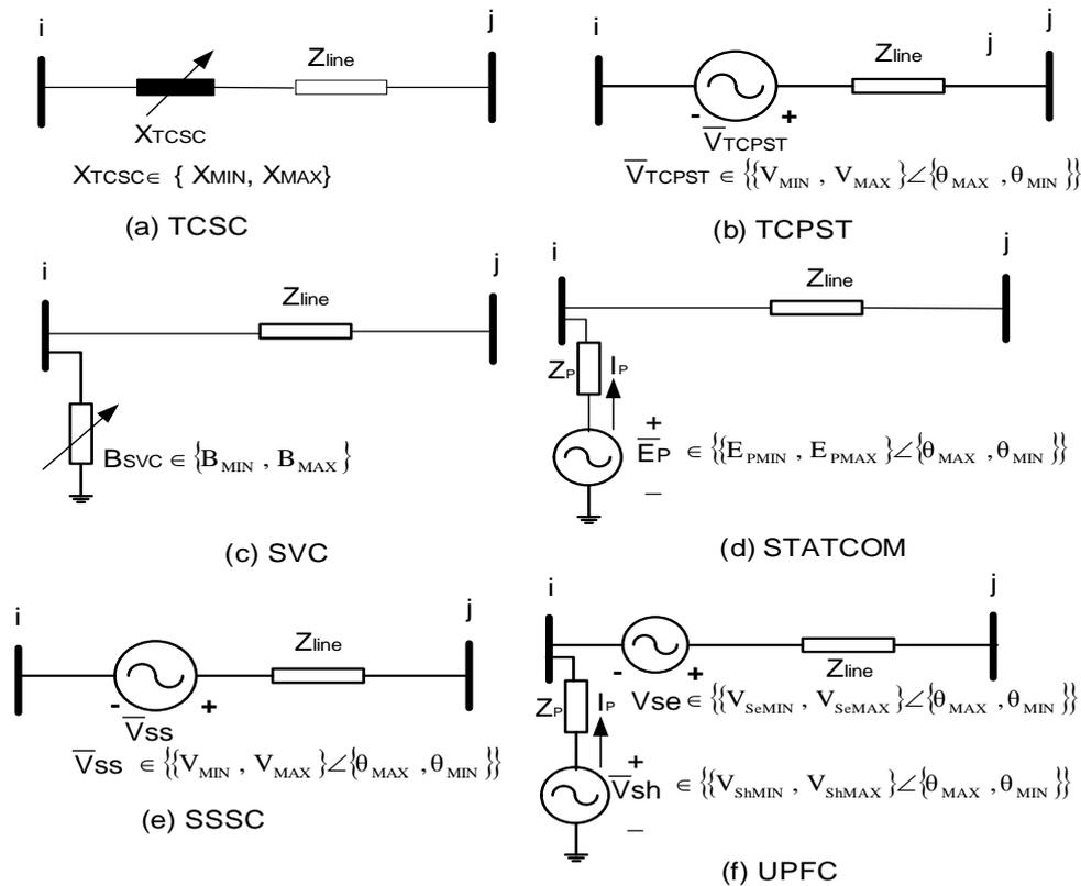
Figure 3: Equivalent Circuit of Various FACTS Devices
