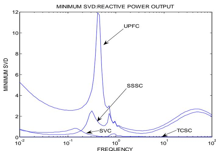
Figure 8: Minimum SVD for Reactive Power Feedback
